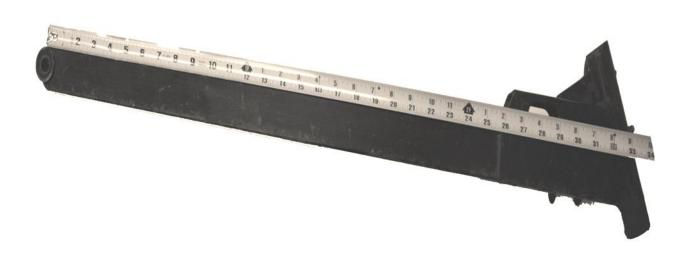
Dimension is from center line on rear trailing arm mount, to reference mark or grease zerk depending on if using OEM or aftermarket trailing arm. The length required is 33 inches.
